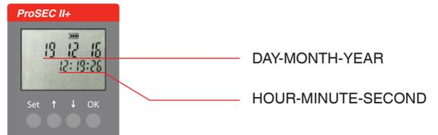
After time/date is set, an option for CLEARING ALL DATA appears. Choose option Yes or No with the UP(↑) or DOWN(↓) arrows and confirm by pressing OK.
