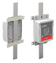
ProLEC Basic is a basic lightning current sensor. It senses and logs lightning discharges flowing through the down-conductor. The ProLEC Basic is capable of measuring and withstanding currents up to 100kA  $(10/350 \mu s)$ .
