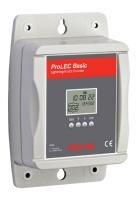
ProLEC Basic is a basic lightning current sensor. It senses and logs lightning discharges flowing through the down-conductor. The ProLEC Basic is capable of measuring and withstanding currents up to 100kA (10/350).
