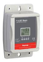
ProLEC Basic is a basic lightning current sensor that detects and logs lightning discharges flowing through the down-conductor. It is capable of measuring and withstanding currents up to 100 kA (10/350 μs).
